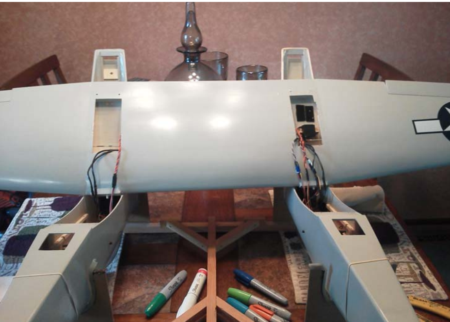
Left: installation of the wing along with all the extensions. Color coded for ease of assembly.
